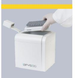
High Speed Rack Reader Delta50 is a one-of-akind camera-based rack reader that can decode 1D rack barcodes and 2D Data-Matrix tube codes.
