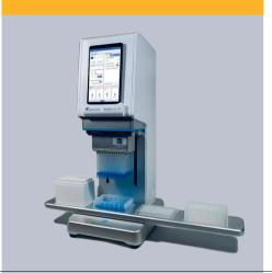
The AutoMATE<sup>™</sup> 96 offers fast, precise 96-channel pipetting for 96/384 well microplates and PCR plates. Features include a touchscreen tablet, 4-position motorized platform, and interchangeable pipette heads (1-1000µL). Includes user-friendly software for seamless setup/operation.
