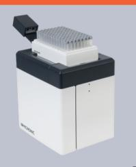
Efficiently read entire racks of 2D Data-Matrix coded tubes in just 3 seconds with the highspeed, camera-based Micronic Rack Reader DR900. Optional 1D Side Barcode Reader reads rack barcodes in only 1 second. Comes with userfriendly Micronic Code Reader Software for seamless lab integration, included at no extra cost. AutoMATE<sup>™</sup> 96 Microplate Pipetting Workstation
