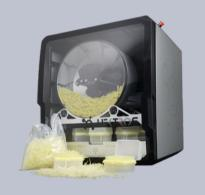
Automates pipette tip refilling, handling up to 1,000 tips per drum in under 30 minutes. Supporting tips from 0.1–1,000 µl and reusable TipBoxes, it saves time, reduces plastic waste, and streamlines your lab's workflow.
