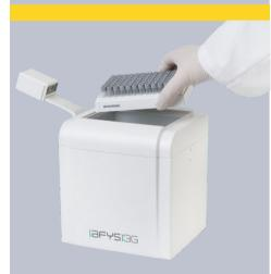
The High-Speed Rack Reader Delta50 is a camera-based rack reader that can decode 1D rack barcodes and 2D Data-Matrix tube codes in less than 3 seconds. Eco-Friendly Choice (EFC) Range
